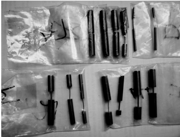
Figure 8.1: Phantoms of copper, different diameters and different length of the "stenoses".
