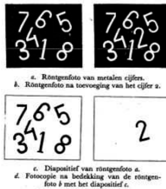
Figure 17.1: Principle of subtraction as published by Ziedses des Plantes [3].
