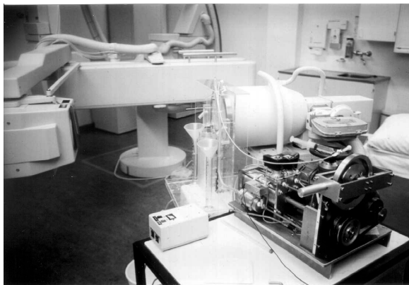
Figure 8.9: Overview of the experimental set-up to measure coronary flow, consisting of the pump system and X-ray equipment.
